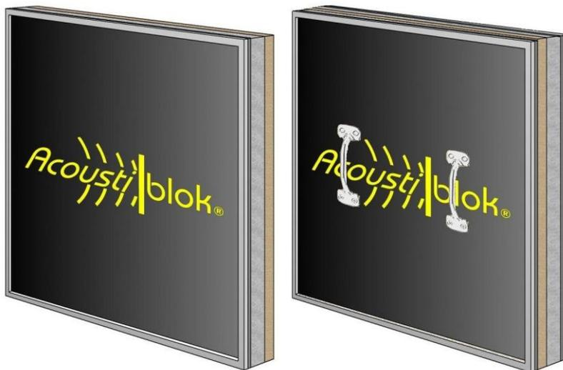
The above graphic shows a way to create a window plug that is very effective by incorporating Acoustiblok and simple construction materials into a removable solution for studio windows. This requires two layers of Acoustiblok, 6lb. fiberglass duct board,  $\frac{3}{4}$  plywood or  $\frac{3}{4}$  HDF, 1 pr. of handles.
